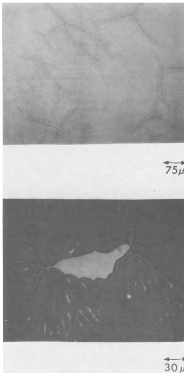
Fig. 2. Micrograph of "frosted" unirradiated regions of developed film showing development of microcracks.
