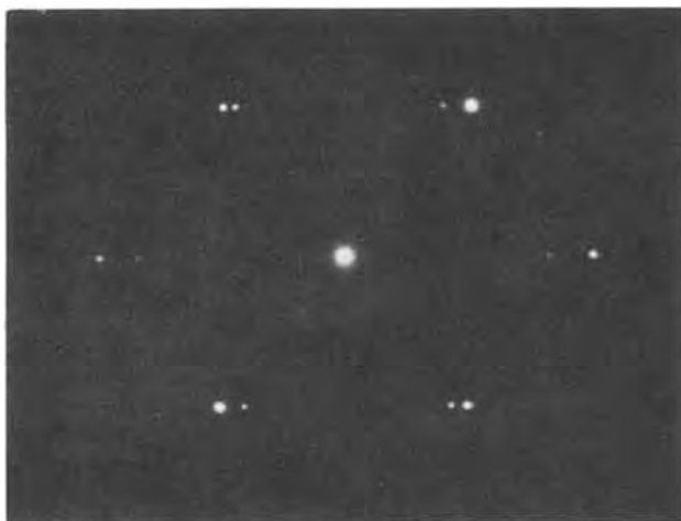
Fig. 5. (a, above left) Diffraction pattern of a film of CdSe grown on (110) Ge at 440°C. This is the pattern obtained when the film is tilted slightly off the exact (110) orientation. (b, above right) Bright field transmission electron micrograph of the same film.
