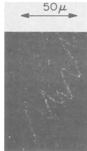
Fig. 3. Microprobe photograph of another location of specimen in Fig. 2 where again white areas represent silicide within the metallization.
