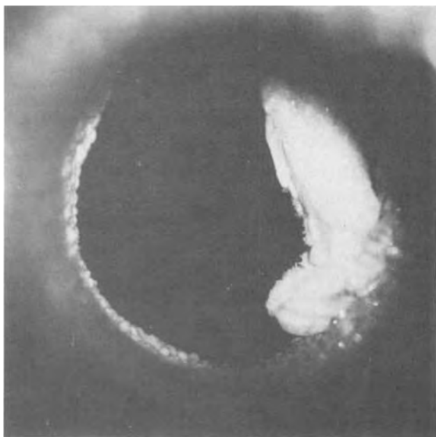
c. Whiskers on surfaces of opaque deposits obtained at 1200°C.
