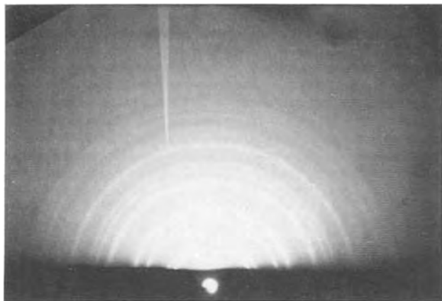
Fig. 1. A 60 kV RHEED pattern of the product film formed on \text{TiO}_2 during exposure in sensitizing solution A.
