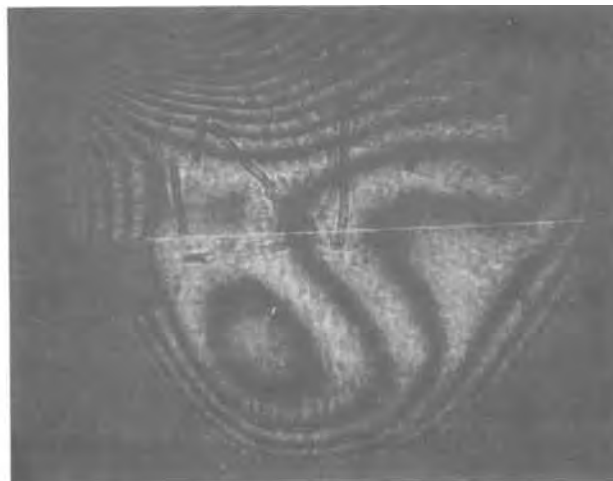
Fig. 5. Topograph of a slice adjusted before beveling (a, left) and after beveling (b, right). A small rectangular patch of paper glued on the slice, serves as a starting point for the photographic analysis and spreading resistance measurements.
