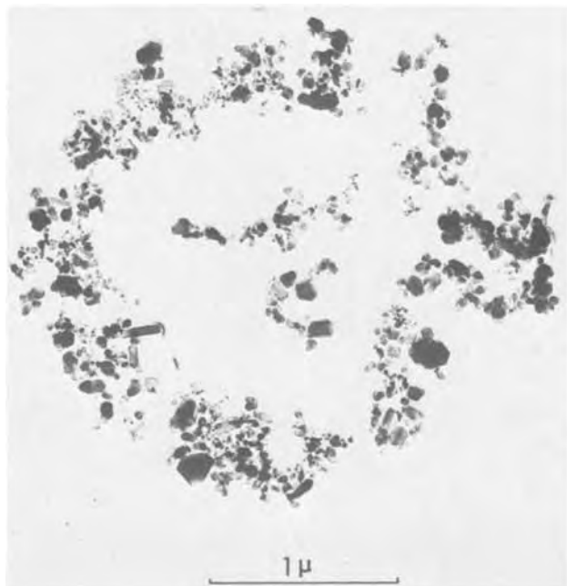
Fig. 8. Electron micrograph of B_4C . (X40,000).
