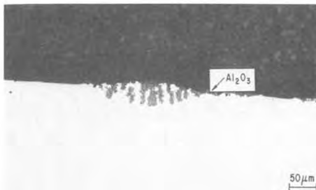
Fig. 16. Section of Ni-30 Al coupon after 5 hr immersion in 1g \text{PbSO}_4 at 900^\circ\text{C} in 0.1% \text{SO}_2 -76% \text{O}_2 - \text{N}_2 atmosphere.
