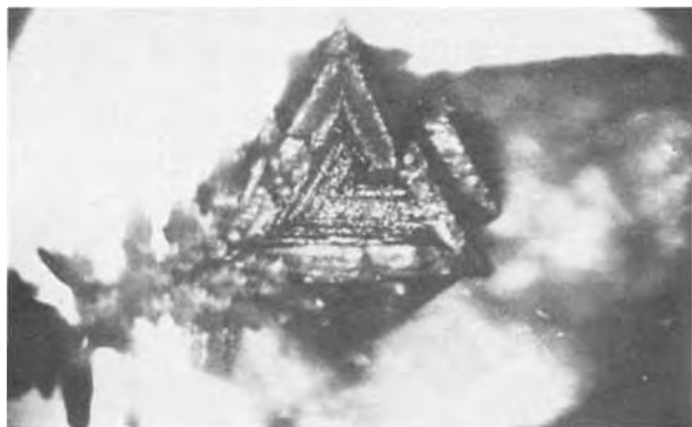
Fig. 2. Hopper growth on (111) face of a crystal ( \times 30 )
