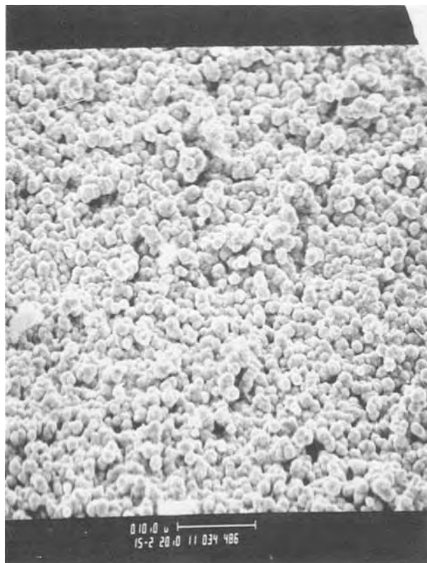
Fig. 18. Scanning electron micrograph of silver deposit obtained at current density of 3.0 \text{ mA/cm}^2 and 12 min. Magnification 1500X.
