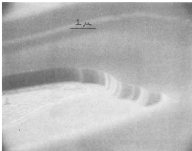
Fig. 8. SEM micrograph of a contact window with ledge removed
