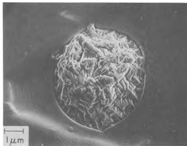
Fig. 4. SEM photomicrograph of Ga droplets located at the bottom of a typical conical etch pit.
