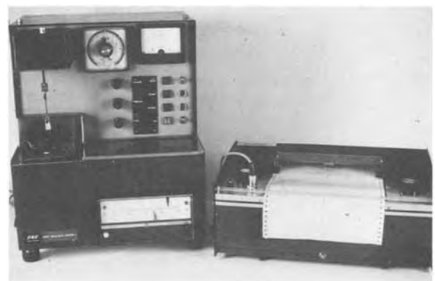
Fig. 14. Commercial apparatus for determination of the wetting time of materials.
