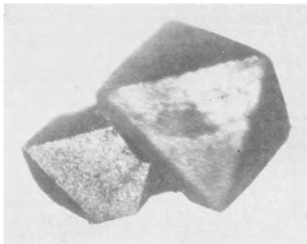
Fig. 1. Single crystal of CdO showing (111) faces. Octahedral morphology ( \times 40 ).
