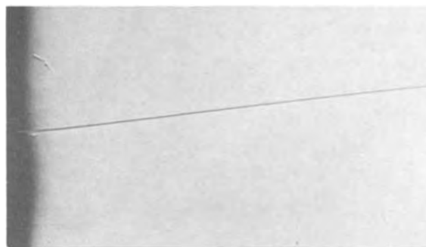
Fig. 15. Dopant segregation discontinuity caused by cooling arrest and thermal soaking during growth in Skylab-IV mission. Magnification 400\times .
