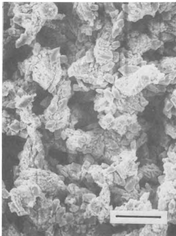
Fig. 3. Coralloid structure in the discharged active material ( \text{PbSO}_4 crystals) after 40 discharges. As seen with the SEM. Scale length = 20 \mu\text{m} .
