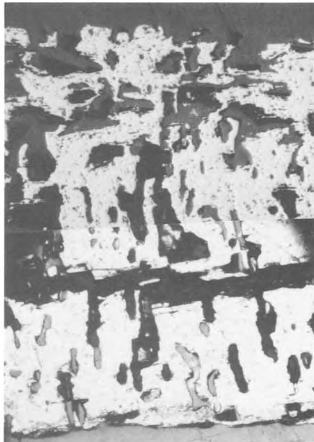
Fig. 6. Selected area of Fig. 5 at higher magnification. The pores in the layer grown on the selenium-exposed face are irregularly shaped while in the original wafer they are perpendicular to the faces.
