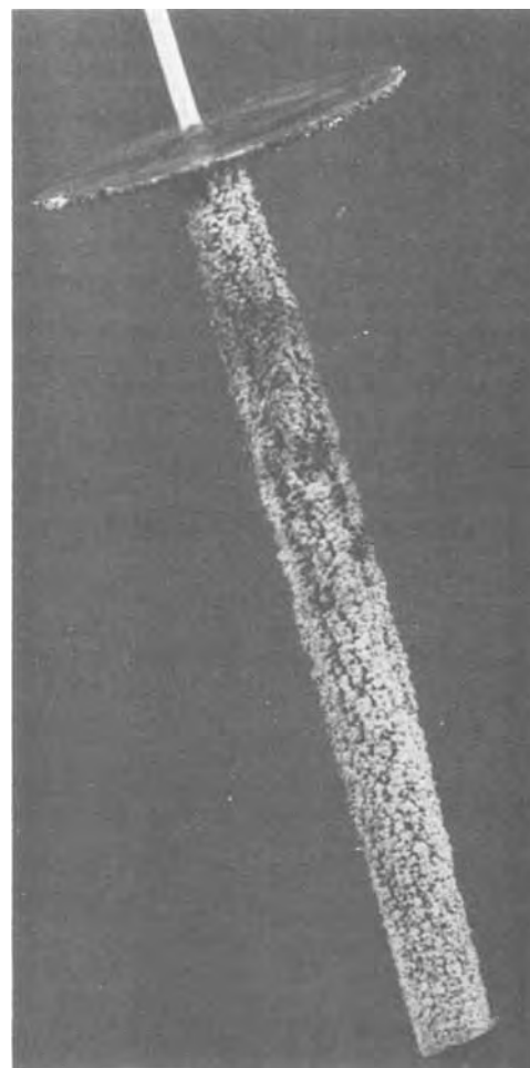
Fig. 2a. Copper cathode with interfacial disk. Top view. Diameter of disk, 2.0 cm
