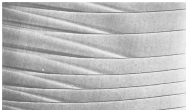
Fig. 20. Rotational striations (narrow lines) in a Te-doped crystal of InSb. Although the pulling rate and the rotation rate were maintained constant during growth, the distance between rotational striations is not constant, indicating that the actual growth rate is not the same as the pulling rate. 150X.
