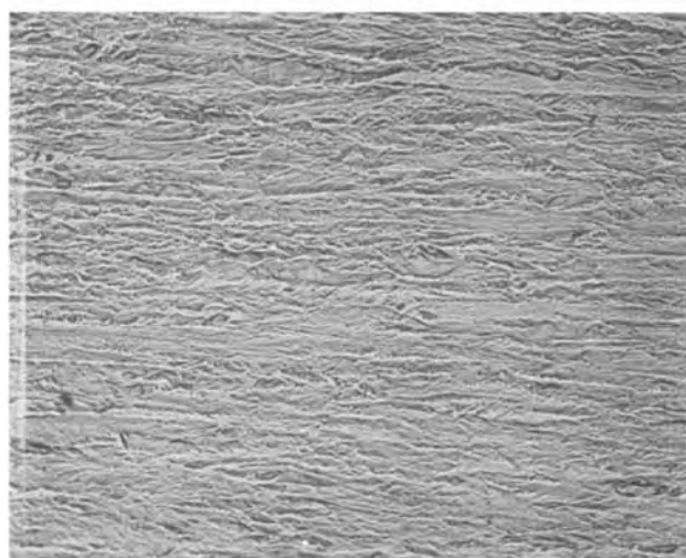
Fig. 6. Microstructures showing the effect of Al inclusion in nickel. Deposits produced at 50°C, 4 ASD. (a, top) Pure Ni, (b, bottom) 0.02 w/o Al inclusion. 740X magnification.
