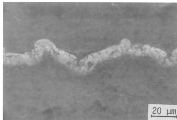
Fig. 9. Cross section of TiN films deposited on quartz at 300°C
