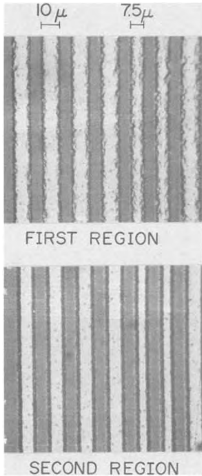
Fig. 2(a) Beveled aluminum patterns for the first and second regions shown in Fig. 1.
