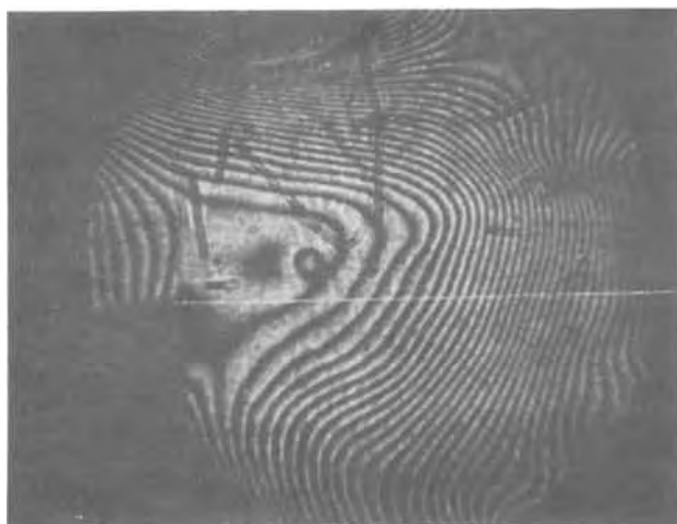
Fig. 5. Topograph of a slice adjusted before beveling (a, left) and after beveling (b, right). A small rectangular patch of paper glued on the slice, serves as a starting point for the photographic analysis and spreading resistance measurements.
