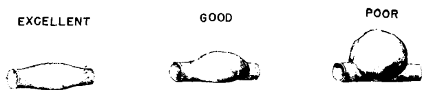
Fig. 8. Wire samples showing solder spread
