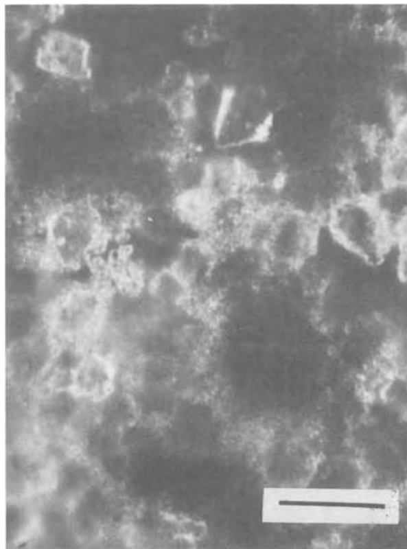
Fig. 9. Same area as Fig. 8, but with polarized illumination. Dark areas corresponding to bright areas of Fig. 8 are in reality slate gray or black, and, as can be seen, are surrounded by a layer of \text{PbSO}_4 crystals. Scale length = 10 \mu\text{m} .
