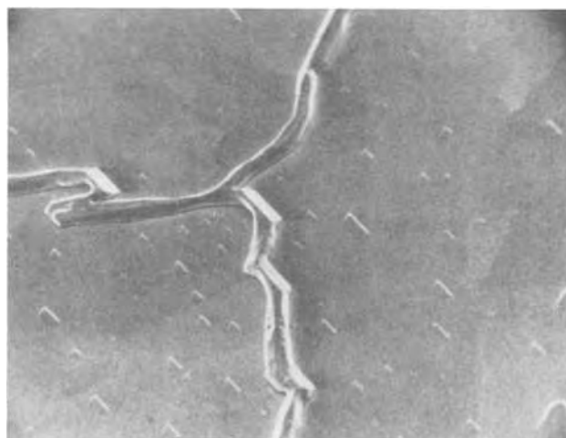
Fig. 8. The back side of the metallization after removal of the Si substrate. The raised features correspond to trenches in the substrate \langle 111 \rangle -Si, and reflect the crystalline nature of the substrate.
