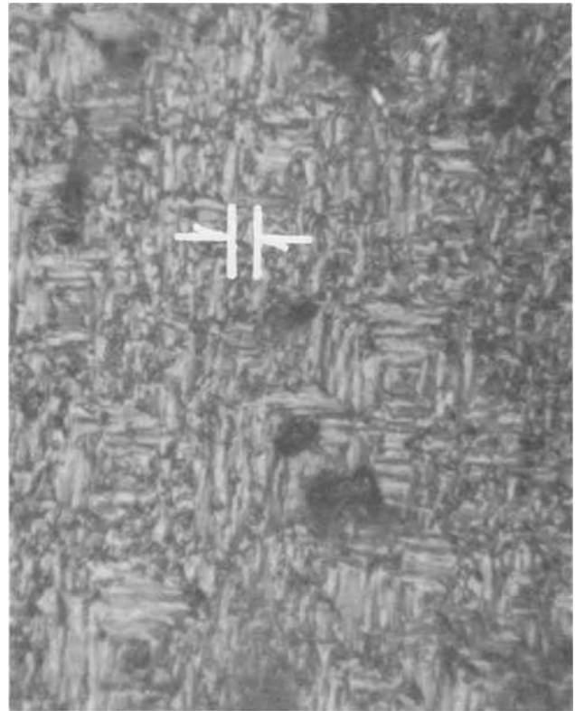
Fig. 2a. Surface of ZnSe epitaxial layer grown from the crushed-crystal source: Nomarski phase contrast; calibration marks correspond to 5 \mu .
