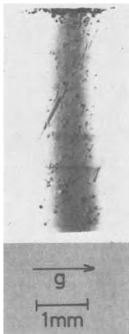
Fig. 8. X-ray projection topograph of tin-doped specimen: concentration of tin 1 \times 10^{19} atom/cm 3 ; t_f = 43\mu .
