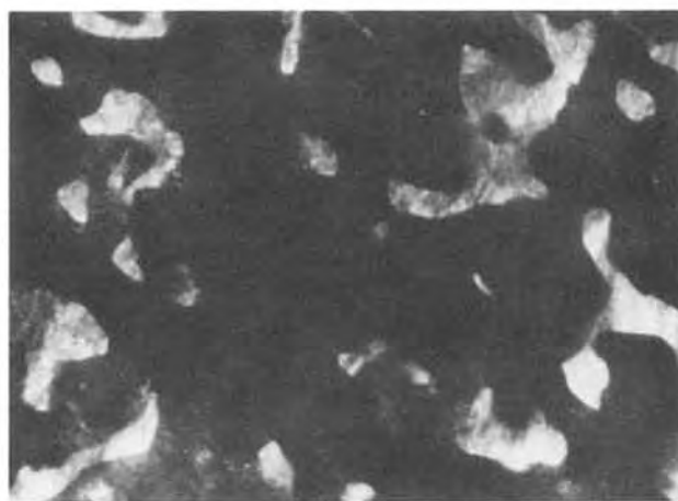
Fig. 5. (a, above left) Diffraction pattern of a film of CdSe grown on (110) Ge at 440°C. This is the pattern obtained when the film is tilted slightly off the exact (110) orientation. (b, above right) Bright field transmission electron micrograph of the same film.
