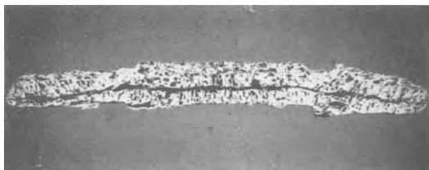
Fig. 5. Polished cross section of wafer after experiment IV. The convex-appearing side (top) was exposed to the selenium vapors.
